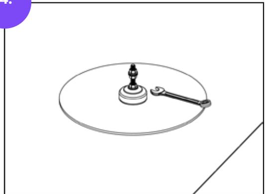
Ensure that the nut and bolt are properly tightened so that all components are securely and watertight fixed.
