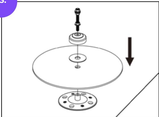
First place the slab and sealing ring over the threaded rod, followed by the cover cap and the knurled nut.
