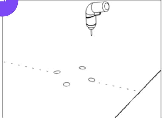
Pre-drill four holes at the marked locations. Then place the plastic mounting plate and secure it with four suitable screws\*, depending on the substrate and insulation thickness.
