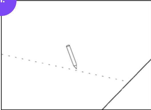
Determine and mark where the mounting anchors will be placed. Take into account the maximum mounting distance of 1.40 meters between the anchors.
