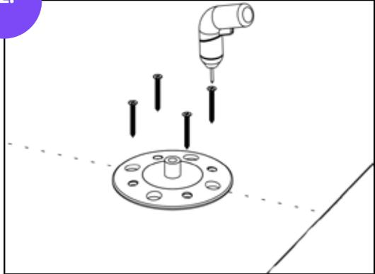
Place the plastic mounting plate in the designated position on the roof. Secure it with four suitable screws\*, depending on the substrate and insulation thickness.
