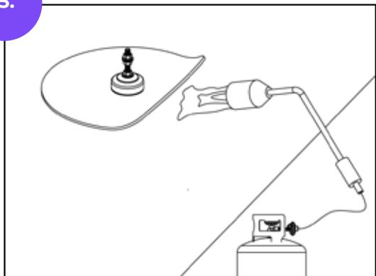
Heat the underside of the slab until the bitumen becomes liquid.
