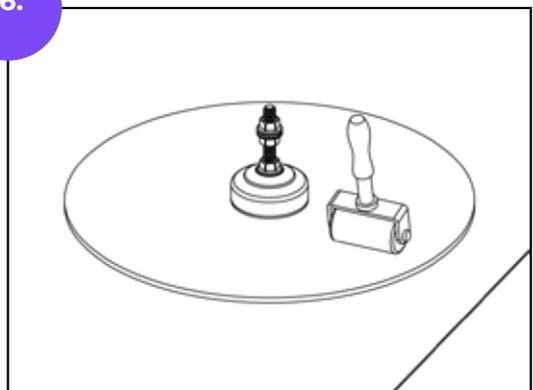
Press the slab firmly with a hard PVC roller to achieve optimal adhesion and sealing.
